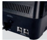
Input/output for tel/fax/ modem line
